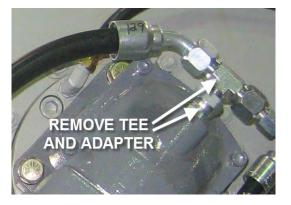
Figure 1: Adapter and Tee Fitting
